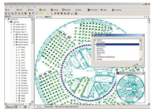
the graphics enable various layers to be displayed - building, lights, sensors, switches, etc - while the system explorer tree shows the architecture and status of the lighting management hardware
